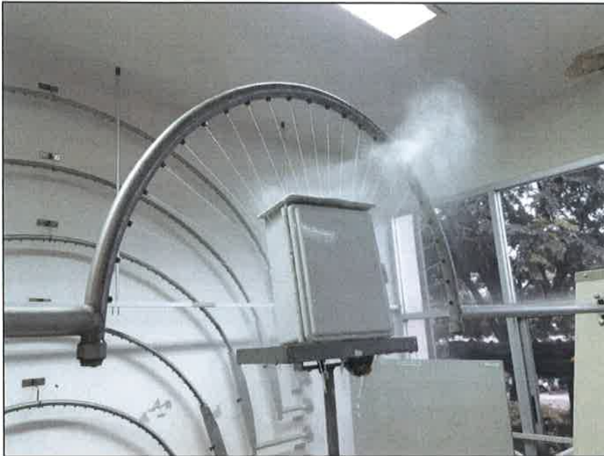
Photo No.5 : IPX4 Water test
