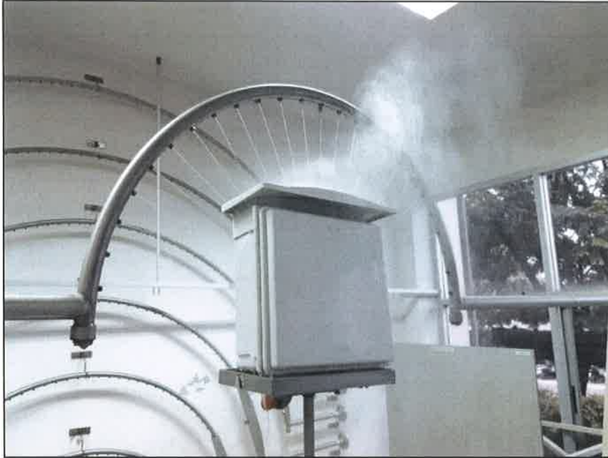
Photo No.5 : IPX4 Water test
